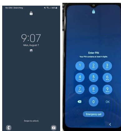
Figure 5: The same Samsung Galaxy A32 5G that was shown in BFU section is now in the AFU lock state. Notice the lack of the “Phone restarted” notification, as well the phone and camera buttons now enabled. The passcode message no longer specifies the device is in BFU mode.
