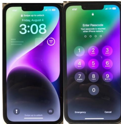
Figure 2: iPhone 14 that is in the BFU lock state (Notice the camera button, lock screen widgets, and Wi-Fi features are disabled, as well as the unique passcode message)
