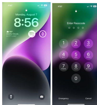
Figure 4: The same iPhone 14 that was shown in BFU section is now in the AFU lock state. Notice the camera, lock screen widgets, and Wi-Fi features are now enabled. The passcode message no longer specifies the device is in BFU mode. A screenshot was able to be taken of both the lock screen and passcode screen.
