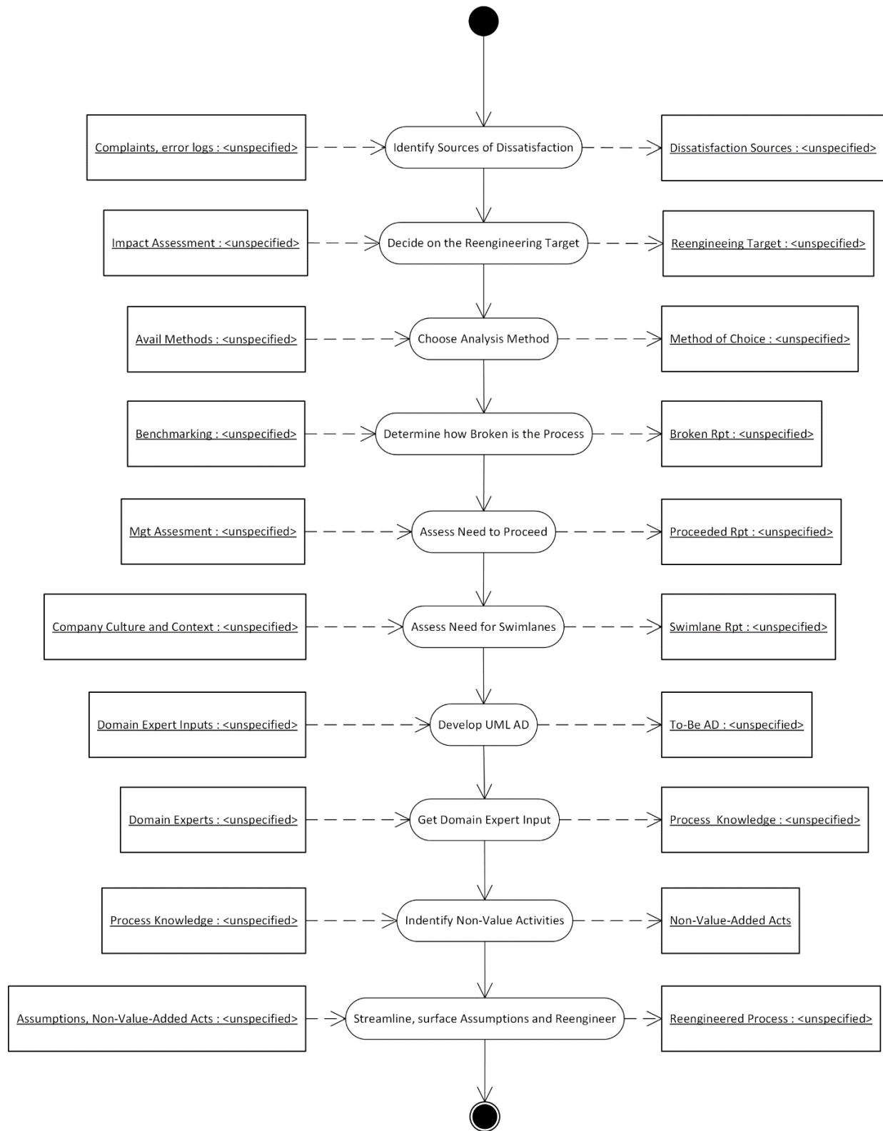
Figure 2: UML- BR Method shown as Activity Diagram
